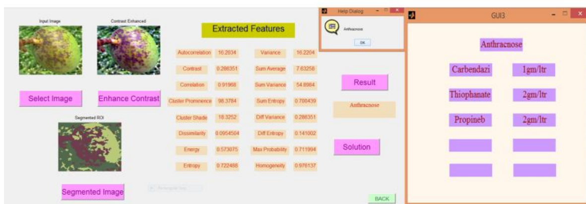
Fig. 7 Anthracnose disease detection on mango fruit
