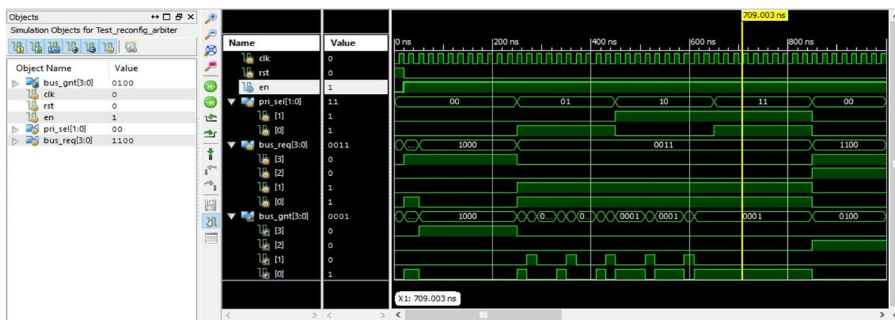
Fig 8: simulation waveforms for lottery bus.
