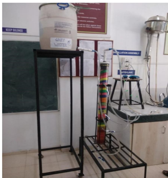
Fig 3 upflow packed bed aerated reactor actual setup
