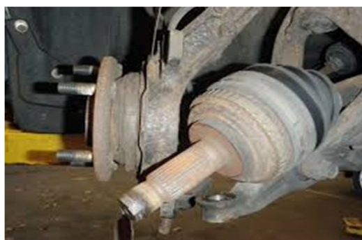
Fig :- IV b )Front Axle failure
