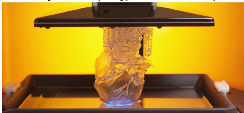
Fig1. printing process with vat and build plate [source: newpro3d.com]
