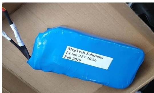
Fig. 3 Lithium Ion Battery
