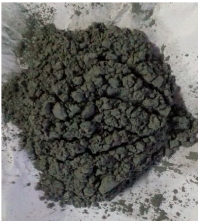
Fig: 2 Preheated cotton shell ash (CSA)
