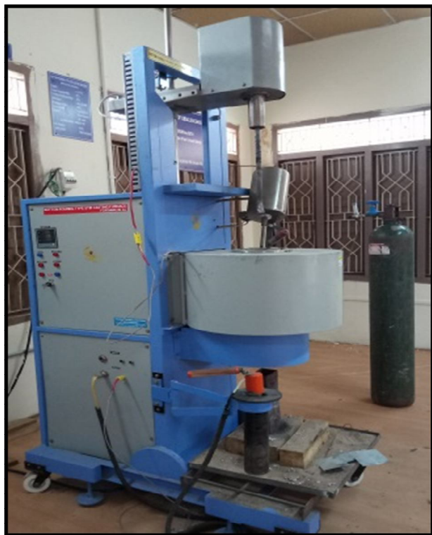
Fig: 4 Stir casting machine
