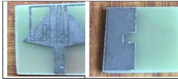
Figure 3: UWB antenna fabrication block
