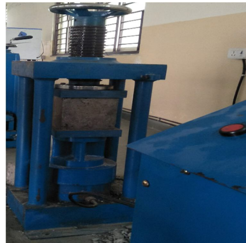
Fig.4 Compressive Strength Testing of Cube specimen
