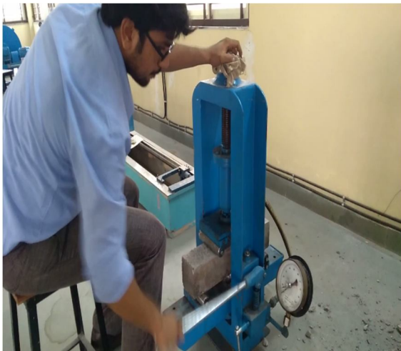
Fig.3 Flexural Strength Testing of Beam Specimen
