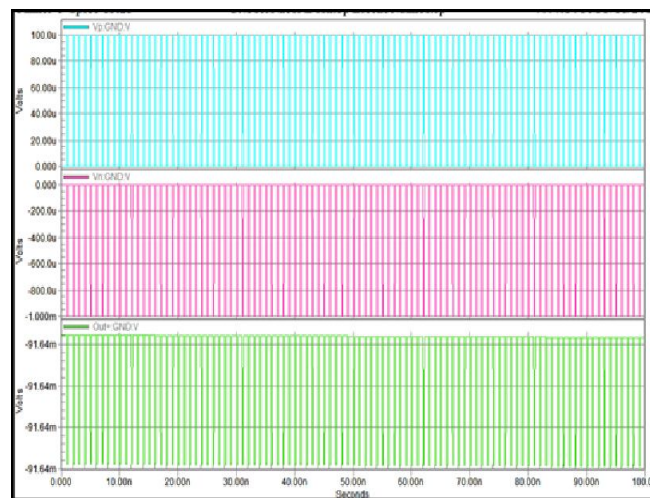
Figure 5: Simulation Waveform of Neural Amplifier VDTA using DTMOS
