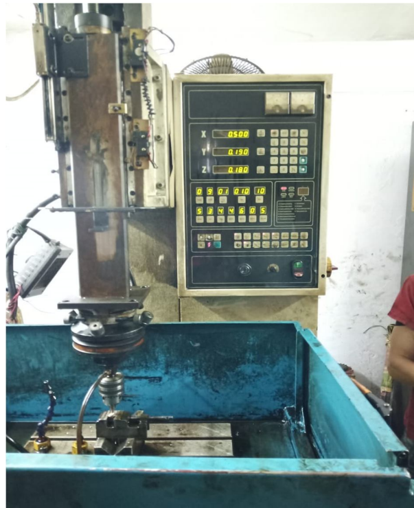
Fig. 1 Setup of EDM for experiments
