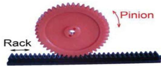
Fig no. 4 Rack and Pinion
