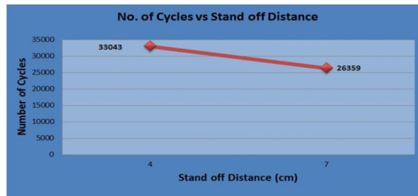
Fig 3.5 Variation of fatigue life with respect to standoff distance
