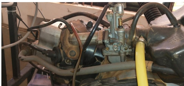
Fig.3: shows LPG connection
