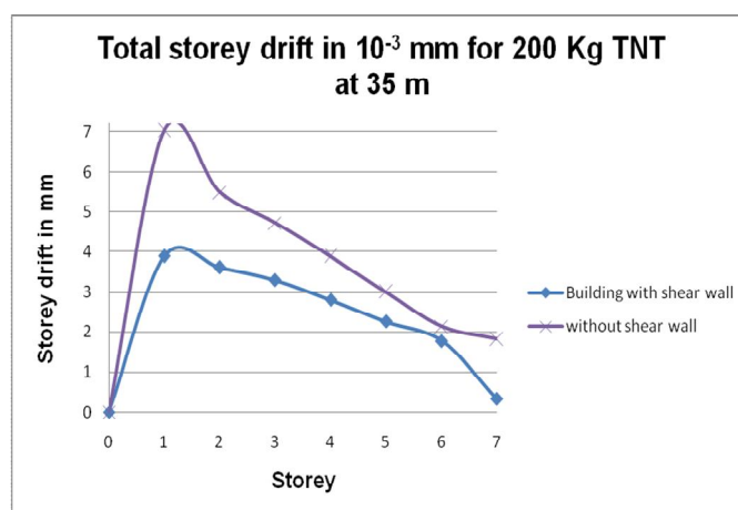
Graph 22: Inter storey drift for a charge weight 200kg TNT at 35m stand-off distance between building with shear wall and without shear wall
