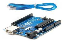
Arduino is an electronic device which is used to read inputs or commands and convert it into output. It helps a user to understand and make it easy for hardware and software to use. By burning the code into Arduino will help the user to move the object according to the command.
