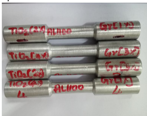
Fig 2 Tensile Test Sample preparation
