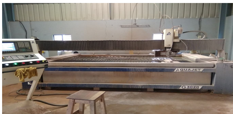
Fig: 1 Abrasive Water jet machining Process Setup
