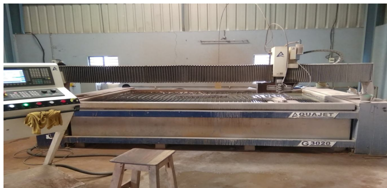
Fig: 1 Abrasive Water jet machining Process Setup
