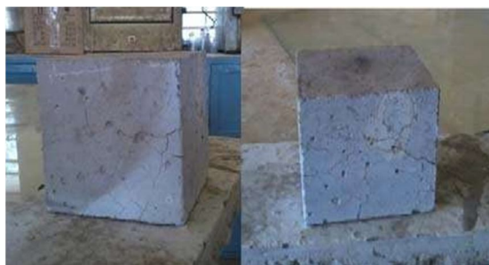
Fig. 4.2: Concrete specimens subjected to 900°C
