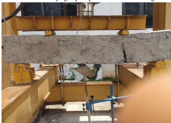
Fig. 11 crack in the specimen
