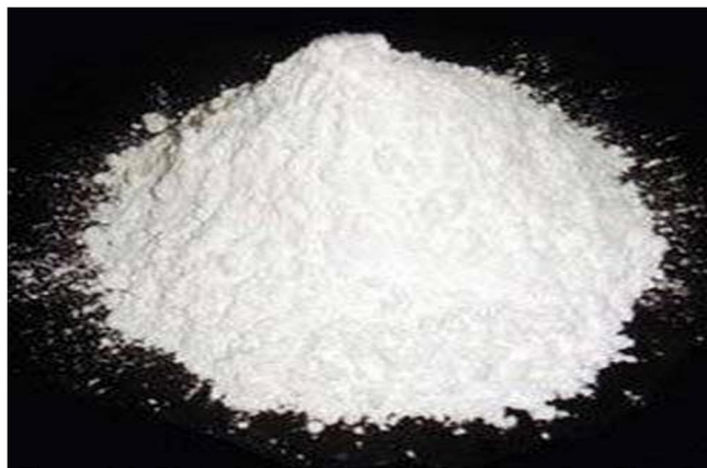
Figure 3.2: 70% of particle passing 0.063mm fine Glass Powder.
