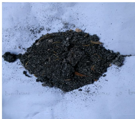
Figure 3.1:70% of particle passing 0.090mm fine Bagasse ash particles
