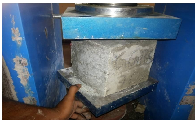
Figure 2 GGBS used Concrete under compressive test
