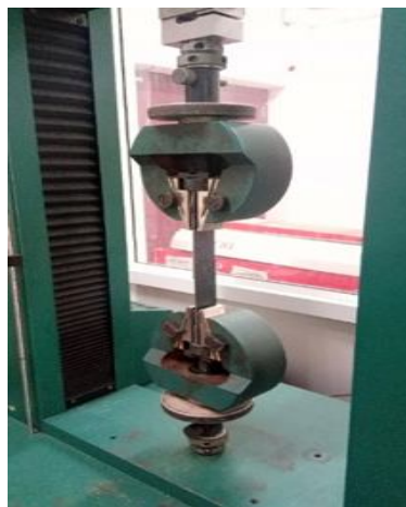
Fig 3.2 Tensile test conducting on Tinius Olsen machine
