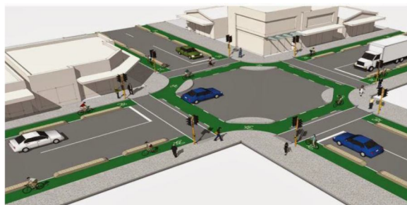
Figure 1.1 .A typical signalized intersection
