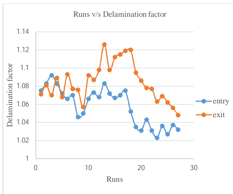
Fig 7 Graphical representation of entry and exit of delamination factor for CFRP with different percentage of \text{Si}_3\text{N}_4
