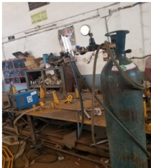
Figure 3: Experimental set up of TIG Welding
