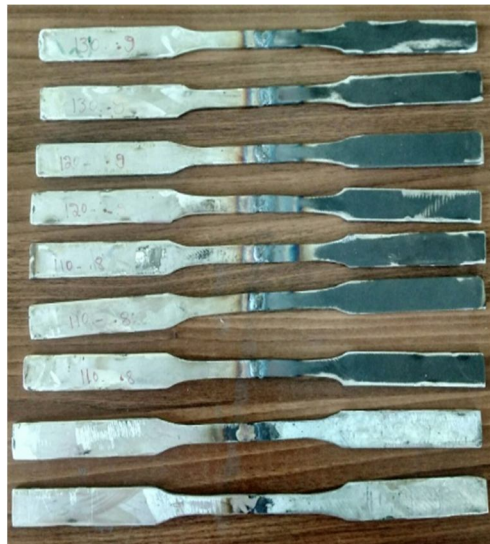
Figure 4: prepared specimen after machining
