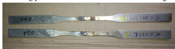
Figure: 2 dissimilar materials welded using TIG welding
