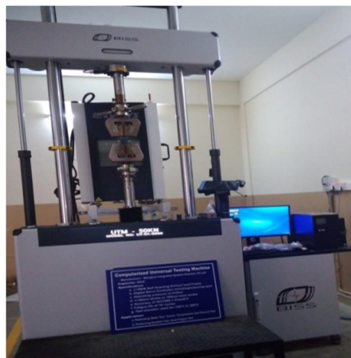
Figure 6: UTM Tensile Testing M/C
