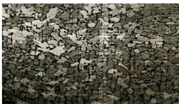
Figure 16 : Microstructure of Parent Zone 500X
