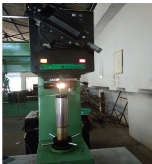
Fig 5: Vickers Hardness Tester Machine
