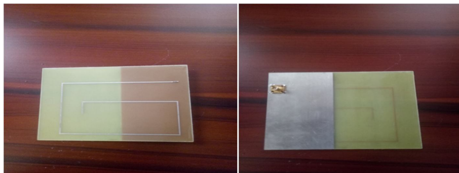
Fig 2: Proposed Near-Field PCB Antenna [Spiral dipole antenna]
