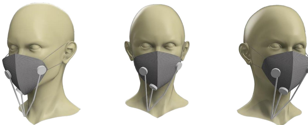
Fig. 3 special design mask with muscle/emg sensor
