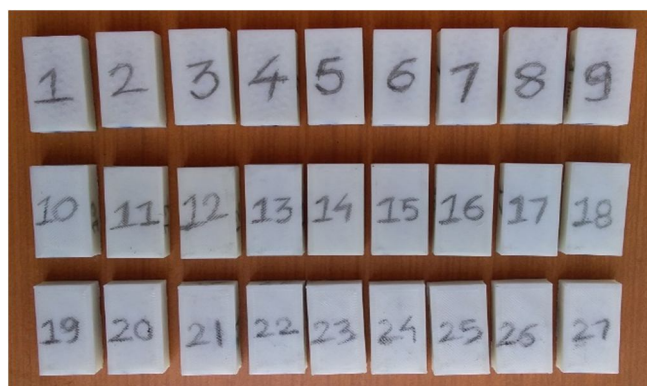
A. Top view of FDM parts
