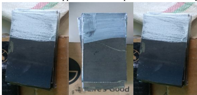
Fig.2. Samples coated with SiO_2 , Al_2O_3 , ZnO flux
