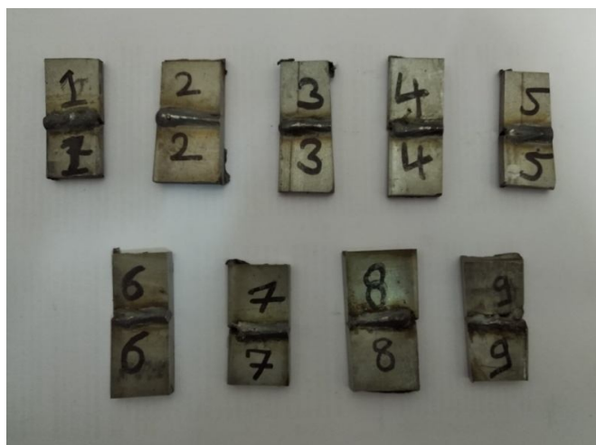
Fig.3: Based on L9 orthogonal array 9 samples for Hardness test
