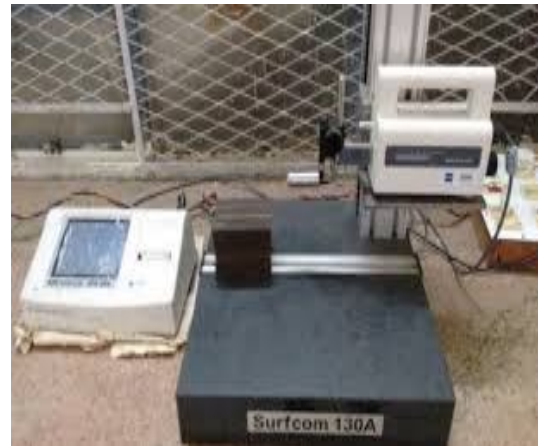
Fig 2.4: Surface roughness measuring instrument (Surfcom 130A)
