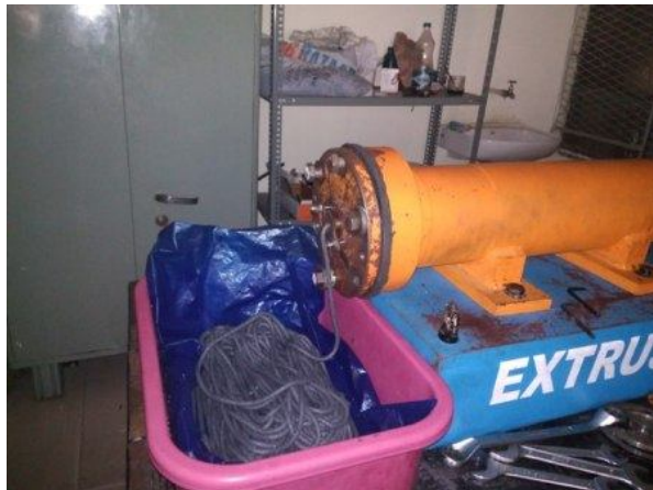
Fig 2.3: Extrusion honing process
