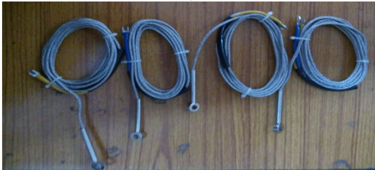
Figure 4:- J-type (Button type ) thermocouples
