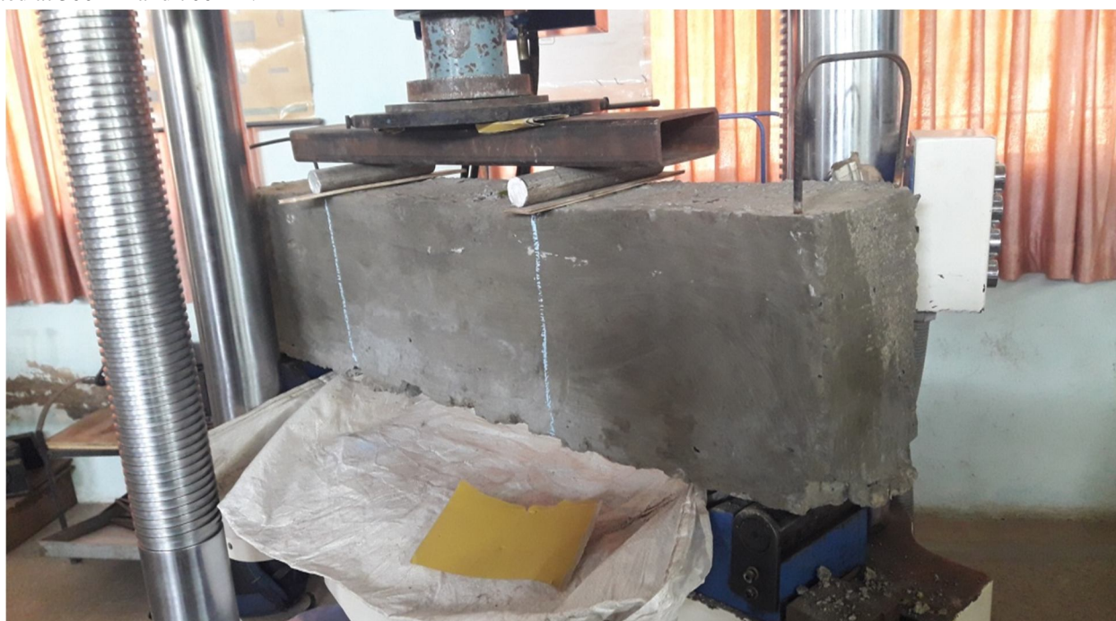
Figure-4. Two point loading test set-up.
