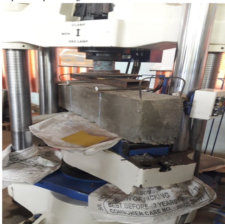
Figure-7. Test beam fixed on UTM assembly.
