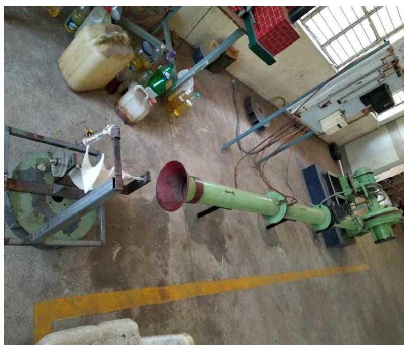
Figure 5 Turbine model in front of Centrifugal blower test rig
