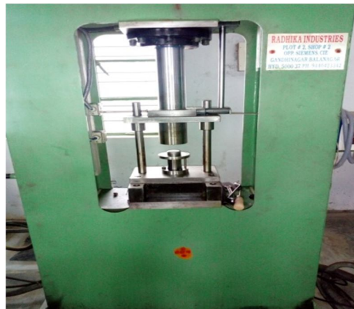
Fig: 4 deep drawing experimental machine.
