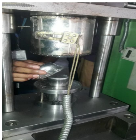
Fig: 9. Experimental Setup used for warm deep drawing.
