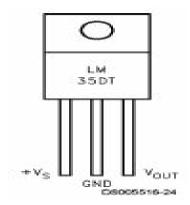
Calibrated directly in  $^{\circ}$  Celsius (Centigrade). Linear + 10.0 mV/ $^{\circ}$ C scale factor. 0.5 $^{\circ}$ C accuracy guaranteable (at +25 $^{\circ}$ C). Rated for full -55 $^{\circ}$  to +150 $^{\circ}$ C range.Suitable for remote applications.Low cost due to wafer-level trimming. Operates from 4 to 30 volts.Less than 60  $\mu$ A current drain.Low self-heating, 0.08 $^{\circ}$ C in still air.Nonlinearity only  $\pm 1/4$  $^{\circ}$ C typical.Low impedance output, 0.1 W for 1 mA load.
