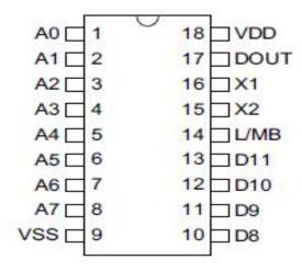
HT12E is an encoder integrated circuit of 2^12 series of encoders. They are paired with 2^12 series of decoders for use in remote control system applications. It is mainly used in interfacing RF and infrared circuits. The chosen pair of encoder/decoder should have same number of addresses and data format.
