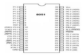
The microcontroller is the heart of this system. The microcontroller used here is 8051 family (AT89C51). It is a 40 pin, 8bit
