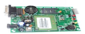
GSM MODEM is a class of wireless MODEM devices that are designed for communication of a computer with the GSM and GPRS
