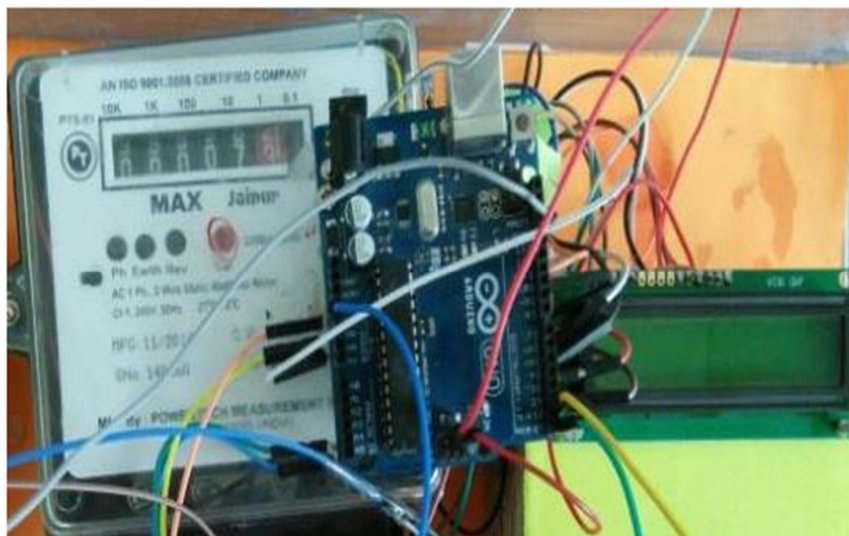
Fig. 2 Energy Meter Execution With, LCD and Arduino
