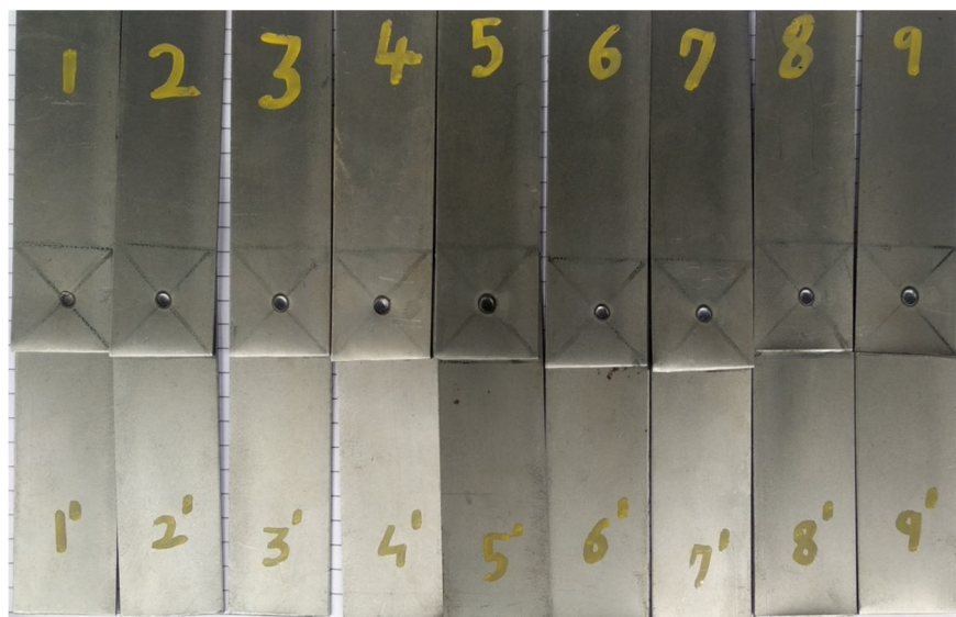
Figure 2.2 Resistance spot welding (RSW) Specimen.
