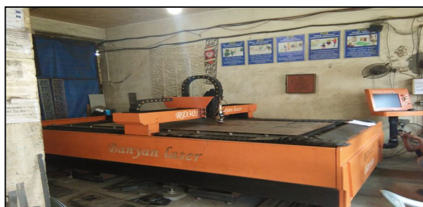
Fig.(6.1): Laser cutting operation for manufacturing super bracket
