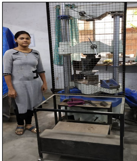
Fig.(6.4): Testing of Manufactured Bracket on UTM
