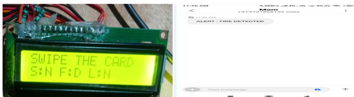
Fig.22 Fire Detection Alert
