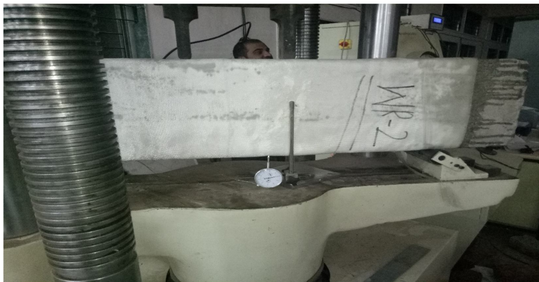
Fig.5. Experimental set-up of RC beams
