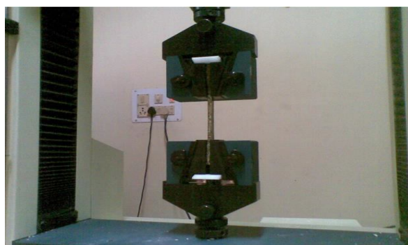
Fig-2: Experimental set up for Tensile Test machine
