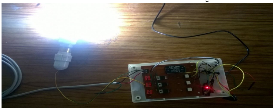
Fig.4 Photograph showing 9w LED bulb remains on when connected to second terminal.
