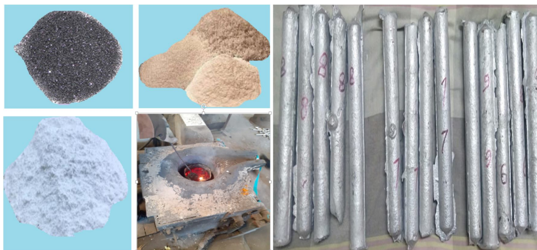
Fig 1.1 stir casting setup and fabricated samples
