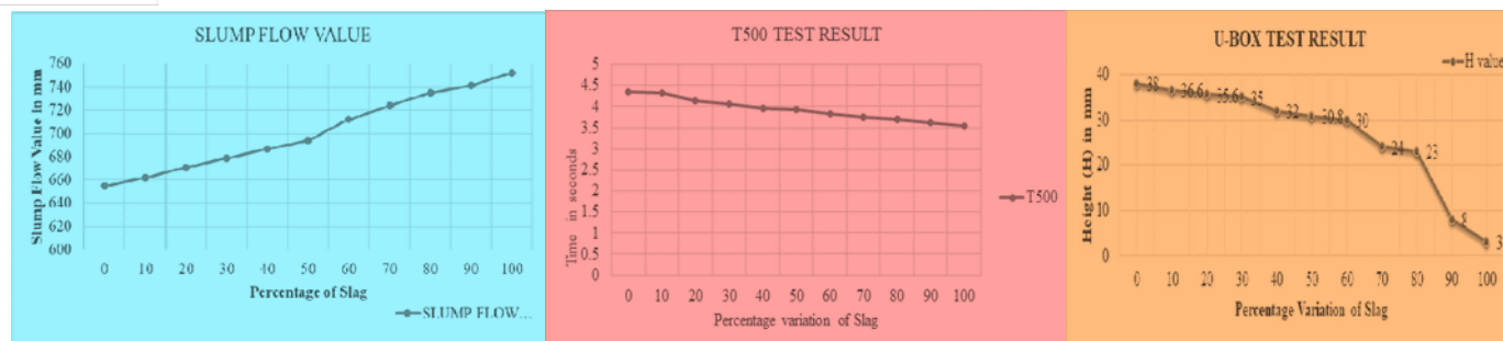
a. Slump-Flow value versus percentage varies of Slag
