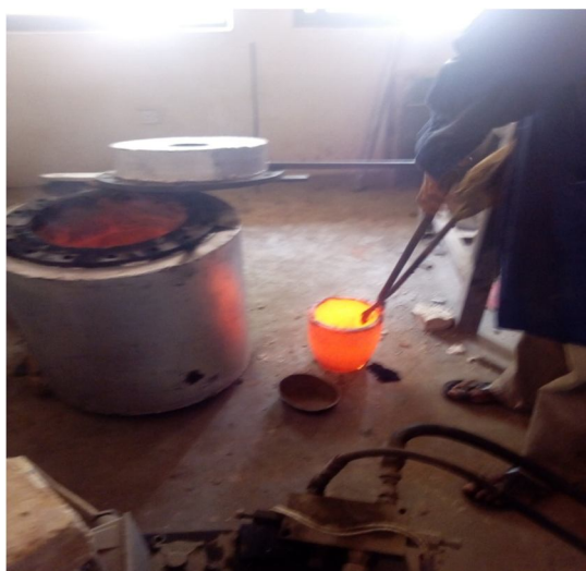
Fig. III Crucible after heating with molten cast iron
