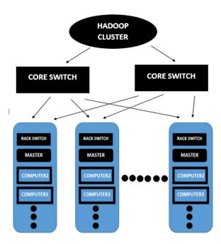
Above is the architecture of Hadoop Cluster [17] consisting of flags, every rack consists of a set of computers and one of the racks consists of a master and these racks uses core switches to communicate with each other. It follows the Rack Awareness algorithm that's all about data storage. According to it the first duplicate of information need to be positioned in the nearby rack and the relaxation of the replicas may be stored on the distinctive far-flung rack.
