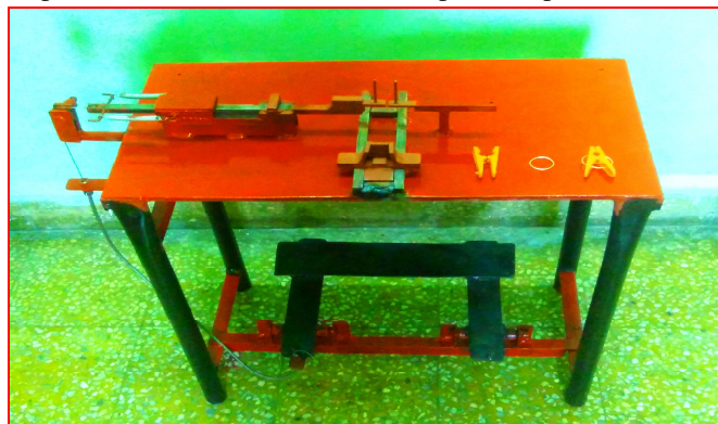
Fig.3 Foot operated Round Ring Cloth Peg Assembly Machine
