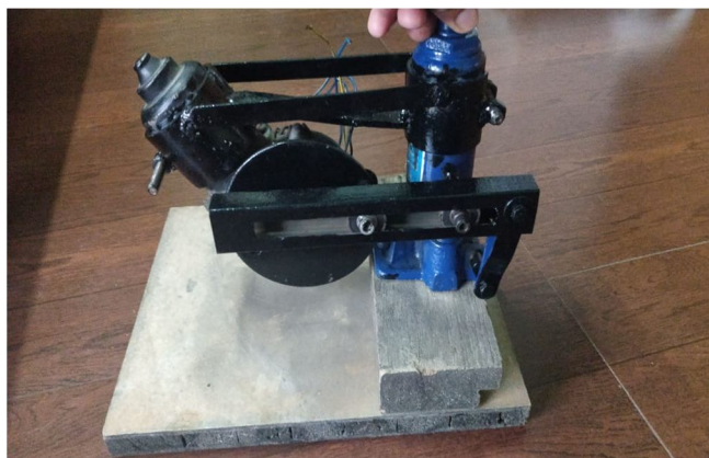
Fig. 2 Designed Hydraulic Jack
